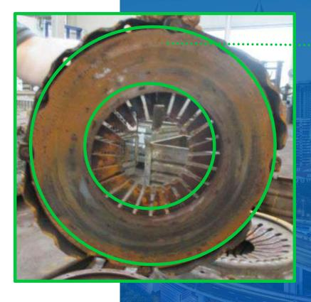
No cracks, not broken Not blue metal "overheated"
