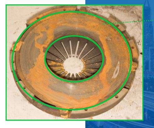
No cracks, not broken Not blue metal "overheated"
